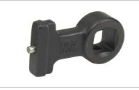
SR adapter '*Crowfoot*' for using interchangeable dovetail attachments on torque wrenches with square drive, e.g. 'Flat Beam'. However, the lever arm must be redetermined in order to calculate the torque achieved.
