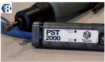
The **PST 2000** uses a combination of three air pressure measurement thresholds and three timers to accurately create a standard conforming fastener. It then compares subsequent fastenings to the standard. The Global Series controller takes the streaming data from the fastening and creates an algorithm from which graphs are created.
