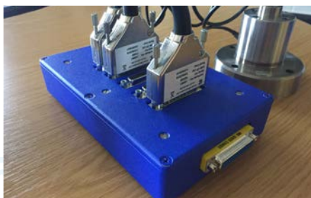
Picture left: Optional Auto Transducer Switch. 5-way sensor switch for Crane 'UTA' or 'Multi' sensors. An LED indicates the currently active transducer. The connected Crane measuring device suggests the most suitable sensor in the display.
