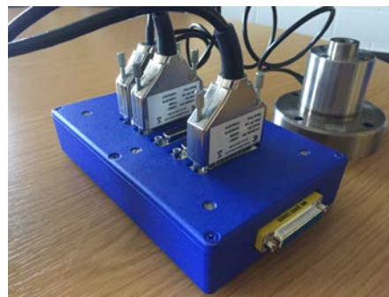
Optional auto transducer switch: 5-way sensor switch for Crane „UTA“ or „Multi“ sensors. An LED indicates the currently active transducer. The connected Crane measuring device suggests the most suitable sensor in the display.
