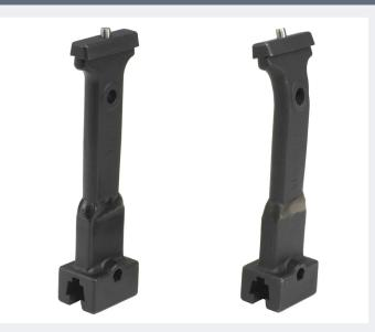
These extensions are designed for use with preset torque wrenches. They can be used to extend the length of the tool if access to the screw location is difficult without the extra length. Due to the changed lever length, the preset click wrench always has to be preset together with the extension and the mounted tool attachment.
