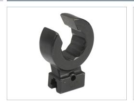
Flare Nut (FN) interchangeable head with Sturtevant Richmont dovetail connector. Cast as a single piece from alloy steel. The manufacturing method provides strength and durability rarely attained by the more common "cut and weld" method. FN flare nut heads are ideal, when:
