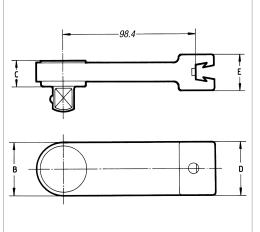
The term 'Common Center Line' means the distance from the base of the dovetail connector to the center of the rotary axis in the interchangeable head.
