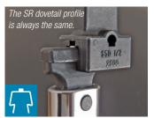
Sturtevant Richmont's micrometer and digital torque wrenches up to 200 Nm capacity are designed for interchangeable heads with 36.5 mm (1 7/16") center line; above 200 Nm capacity, these wrenches are designed for interchangeable heads with 98.4 mm (3 7/8") center line. Otherwise, the scaling must not be applied due to the deviating lever length.
