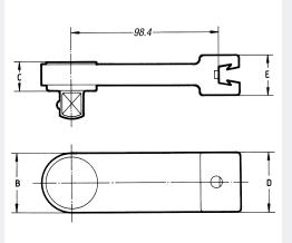
INFO The term 'Common Center Line' means the distance from the base of the dovetail connector to the center of the rotary axis in the interchangeable head. Sturtevant Richmont achieves an exactly constant center distance through the special manufacturing process - from one casting.
