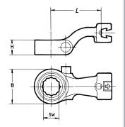
Please note: The torque wrench must be readjusted for each different centre distance!
