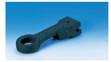
Interchangeable ring spanner head with Sturtevant Richmont dovetail socket. Special version with large centre distance. Can be used with SR torque spanners of the LTC series, SLTC series, SLTC-FM series and CCM series from model 400 Nm rsp. 300 Ft.lb or above.
