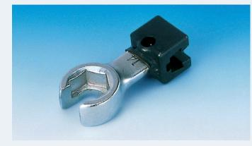
Shoulder flare nut interchangeable head with Sturtevant Richmont dovetail connector. Especially applicable for tightening brake hoses, oil pressure lines or control lines. Suitable for Sturtevant Richmont clicker torque wrench series CCM up to 200 Nm / 1800i / 150 ft.lb, series LTC, series SLTC, and series SLTC-FM.
