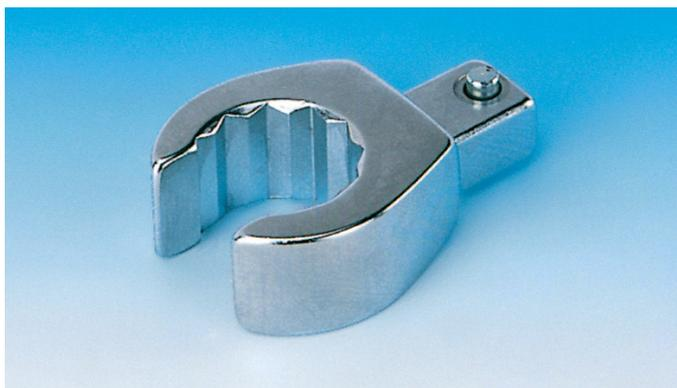
Interchangeable flare nut head with 9×12 mm rectangular insert connector. The attachment is secured by a spring-loaded retaining pin. The load capacity depends on the width across flats and may be less than the capacity of the torque wrench used.
