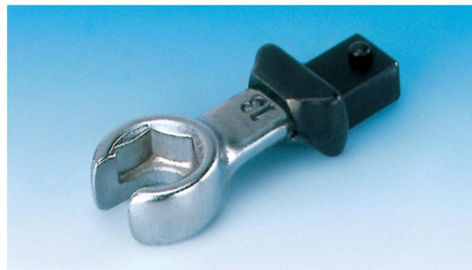
Interchangeable open-end flare nut head with 9×12 mm rectangular insert connector. Custom-made SFN with stop (shoulder) and centre distance 36.5 mm. The attachment is secured by a spring-loaded retaining pin.
