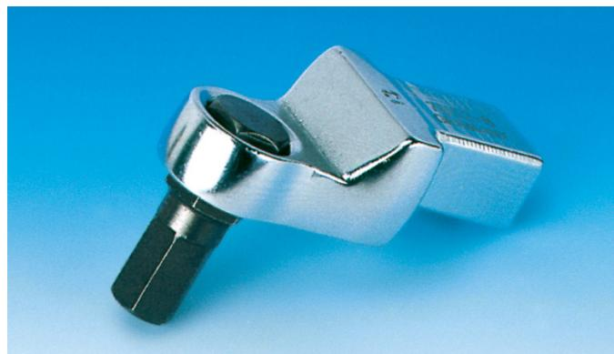
Interchangeable hexagon drive head with 9×12 mm rectangular insert connector. The attachment is secured by a spring-loaded retaining pin. The load capacity depends on the width across flats and may be less than the capacity of the torque spanner used.
