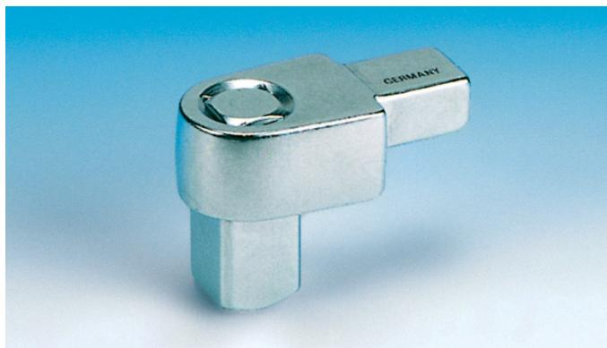
Interchangeable square drive head with rectangular insert connector 9×12 mm resp. 14×18 mm. The attachment is secured by a spring-loaded retaining pin.
