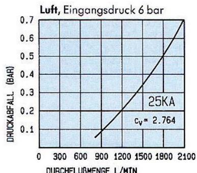
European standard profile hose couplings suitable for compressed air applications with above average compressed air requirements. These European profile couplings have a high flow rate and are available in a variety of configurations and materials that allow for optimal adaptation to the requirements of pneumatic installations.
